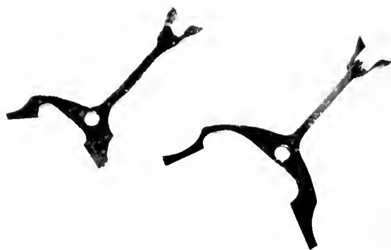
Figure 15. VERGE AND LEVER for an Auburndale timer. The one on the left beats eighths of a second; that on the right beats quarters. (In author's collection.)
